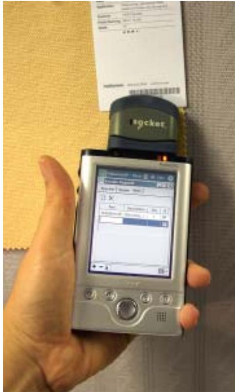
**Figure 3. Pocket PC Running a BBJ Application Scanning Barcodes on Fabric a Swatch.**
