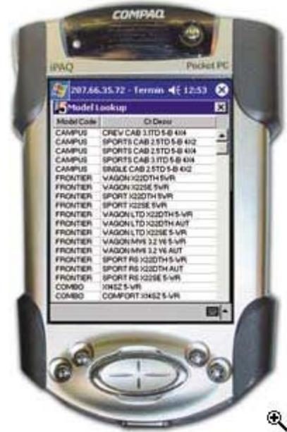
**Figure 6.** Visual PRO/5 application running on a Pocket PC via Terminal Services Client.
